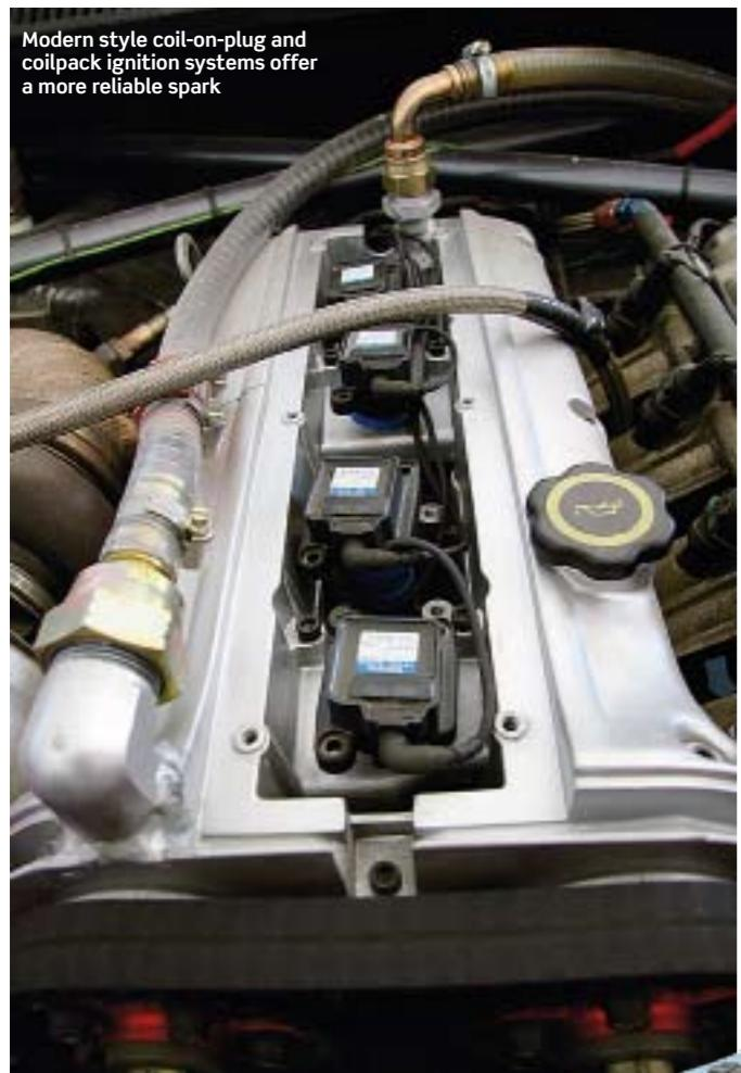
Modern style coil-on-plug and coilpack ignition systems offer a more reliable spark
