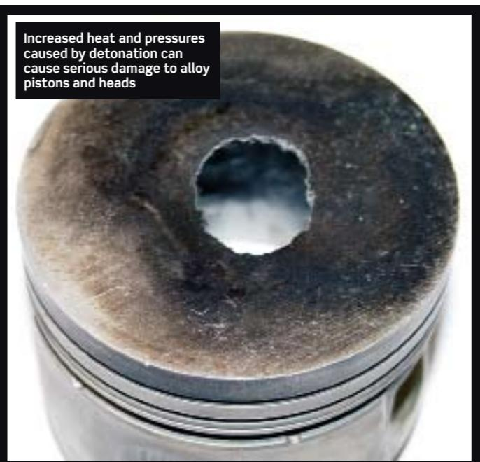
Increased heat and pressures caused by detonation can cause serious damage to alloy pistons and heads
