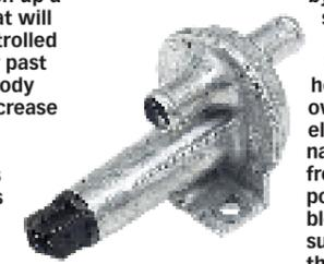
these two ports so it can control how much air is allowed to leak past the closed throttle butterfly, increasing
