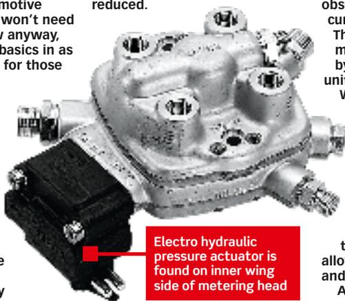
Electro hydraulic pressure actuator is found on inner wing side of metering head
