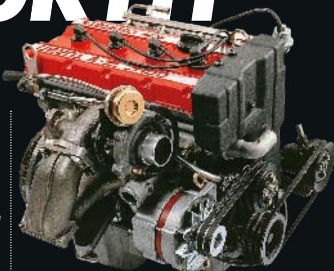
**Stage 5 and above:** After Stage 4, we can lower the compression slightly, beef up the head to block clamping studs and gasket and then add bigger turbos, injectors, fuel pumps, inlet manifolds and cylinder heads to release as much power as most people can afford. With the YB, power available is only a question of, 'How fast can you afford to go?'. **Cost: £4000-upwards**
