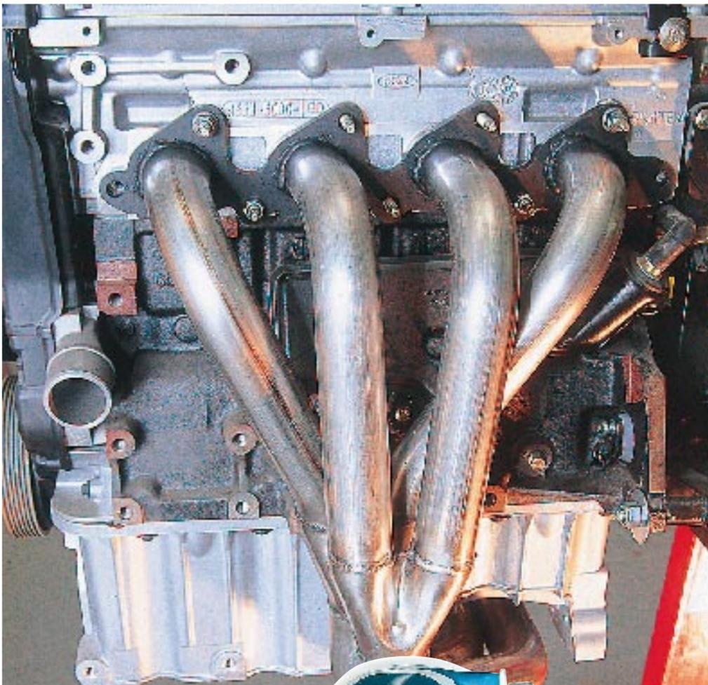
Above. In a perfect world, exhaust gasses would have no restrictions to cause losses, like when a 4-2-1 manifold is fitted to a NA engine
