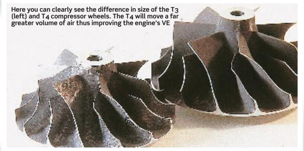
Here you can clearly see the difference in size of the T3 (left) and T4 compressor wheels. The T4 will move a far greater volume of air thus improving the engine's VE
