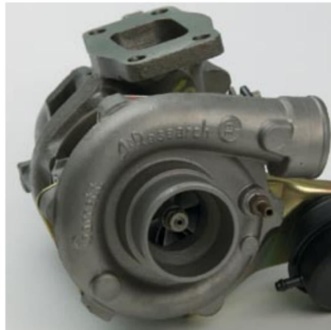
A T3 turbo will produce good power at a given boost limit with relatively low lag, giving good response and driveability
